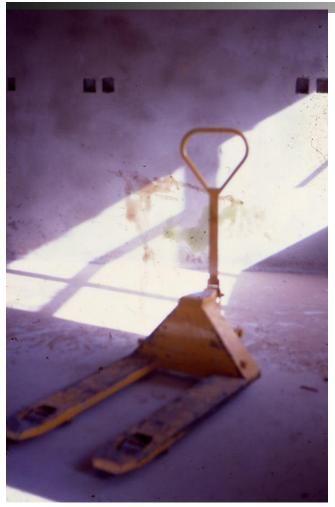
Pallet trolley used to move pallets of bricks at level of use, Port Elizabeth (Smallwood, 1991)
